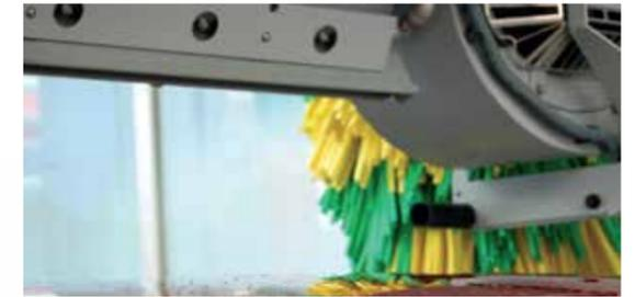
Dryer 12 kW (2 x 3 kW Vertical + 2 x 3 kW Horizontal dryer nozzle plus vehicle scanning and optional diffuser to achieve a better dry on the rear of the vehicle. The best Part is these Dryers are super quiet...Only 71 Decibels
