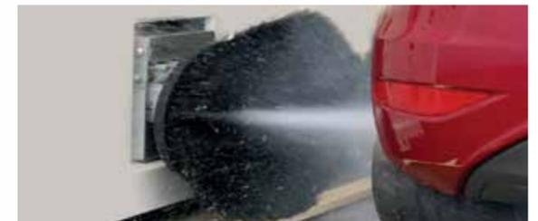
Counter rotating wheel scrubbers constructed of a new stainless steel frame with three vibration absorbing joints! Featuring a new generation of photocells specifically designed for use on our rollover's. They provide greater accuracy and maximum reliability.
